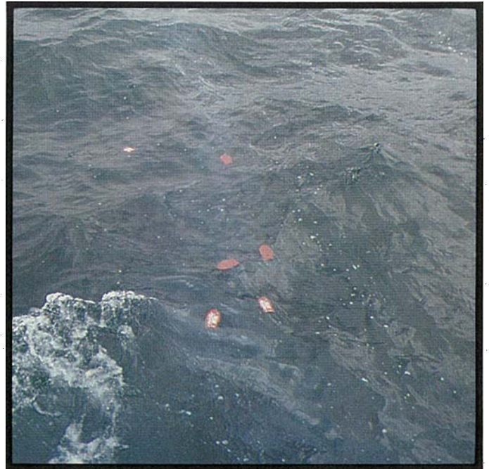
Drift cards: these were released from a boat in batches of 20, and then followed.
