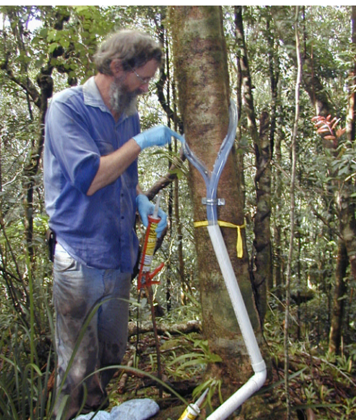
Peter Richardson of CSIRO Land and Water attaches a collar gauge to a tree trunk to measure stemflow.
