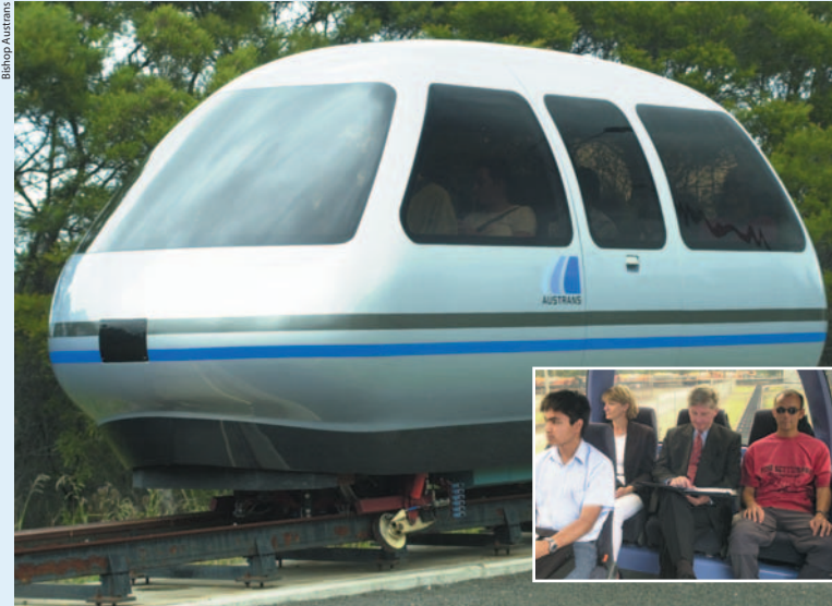
Austrans vehicles are light, quiet, energy-efficient and will travel at up to 120 km per hour. ‘Down the track’, hydrogen fuel cells could be used in place of mains electricity. Inset: The Austrans experience – passengers taking a ride at the company’s test track in Chullora, Sydney.
