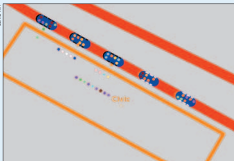
The CSIRO RTSim software simulates transport networks and has proved a valuable decision-making tool. This graphic shows passengers boarding, alighting and waiting at a station, with colours indicating destinations.
