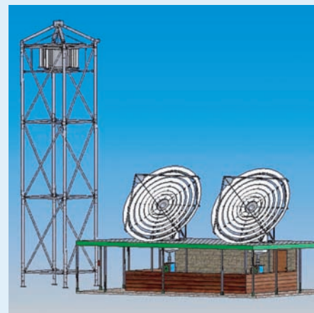
Left to right: CTI’s unconventional wind turbine provides auxiliary power to maintain heat in the salt cell. The turbine uses efficient Venetian-blind-type sails. A two-dish system in situ, similar to those being employed on Fraser Island. Neil Armstrong
