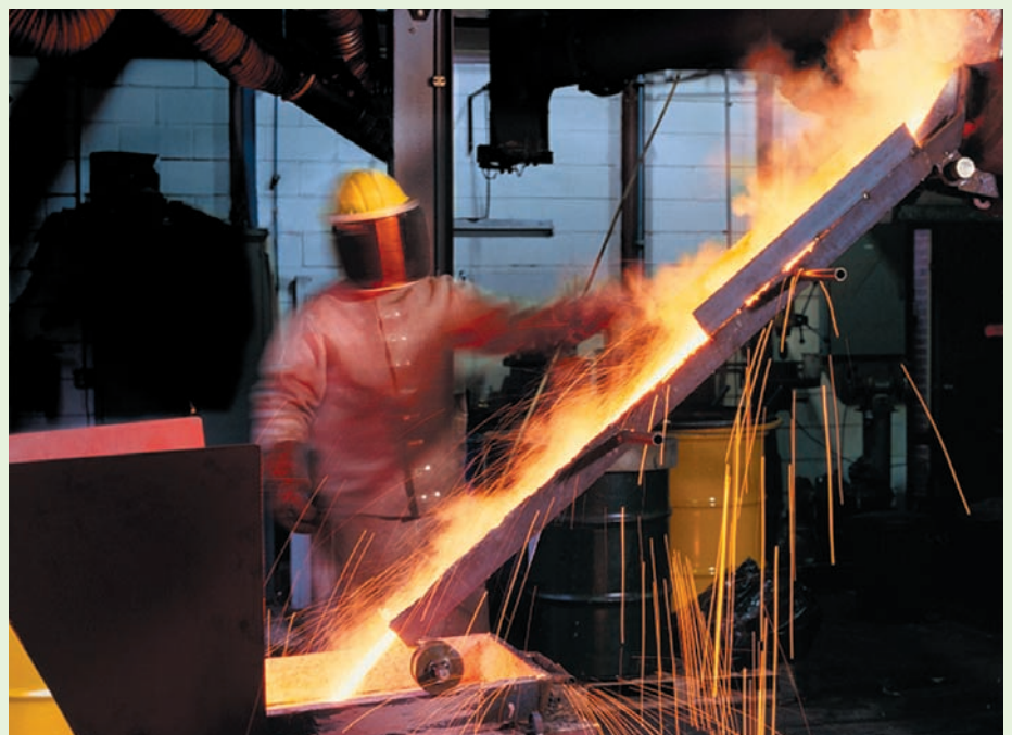
Metals recycling is improving. Molten slag and alloy being poured at CSIRO Minerals’ bath smelting facility. Mark Fergus
