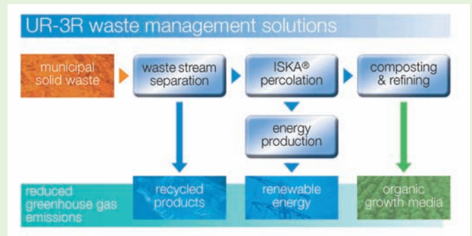
The UR-3R facility receives and processes collected household, commercial and green waste, using a suite of the world's best technologies, to produce a range of recycled products, renewable energy and compost, known as organic growth media. Global Renewables
