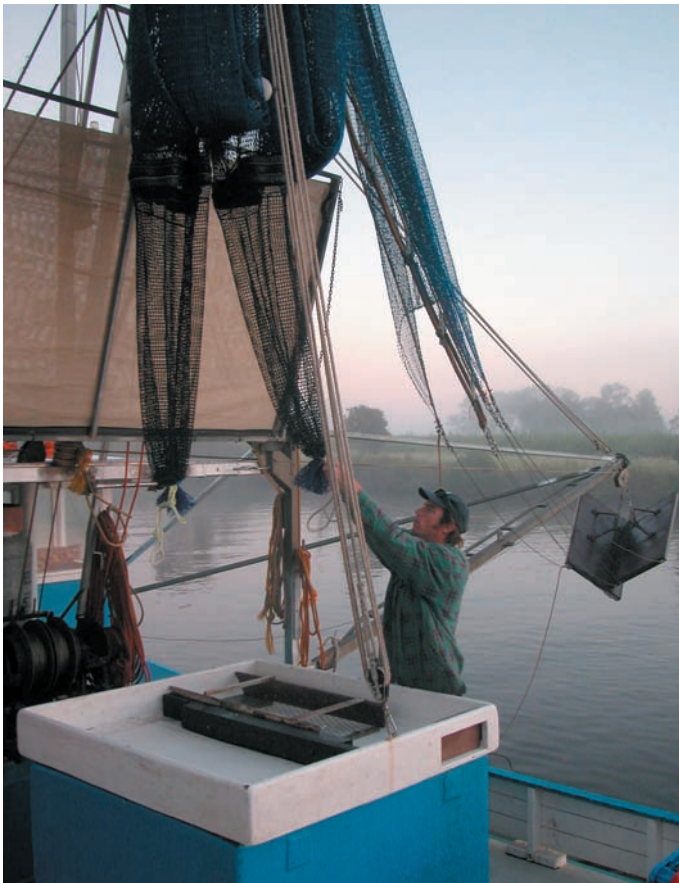
Fisheries technician Michael Wooden checks a 'square-mesh codend' on board a Clarence River prawn trawler. Commercial fishers and scientists are cooperating closely to reduce wasteful bycatch.
