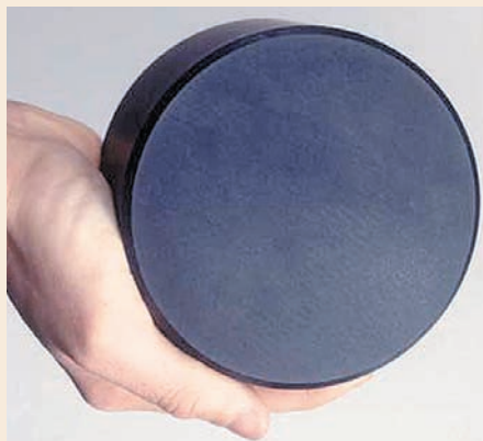
The ceramic synroc was first developed as a way to dispose of surplus weapons plutonium.
