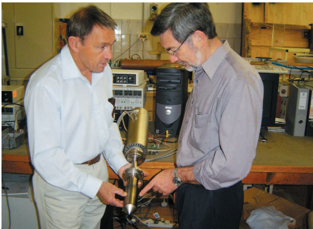
Tony Collings and Paul Gwan examine the transducer and horn that generates the ultrasonic wave in a slurry. CSIRO Industrial Physics
