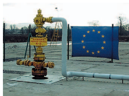
A pumping head at the RECOPOL project site in Poland. CSIRO Petroleum
