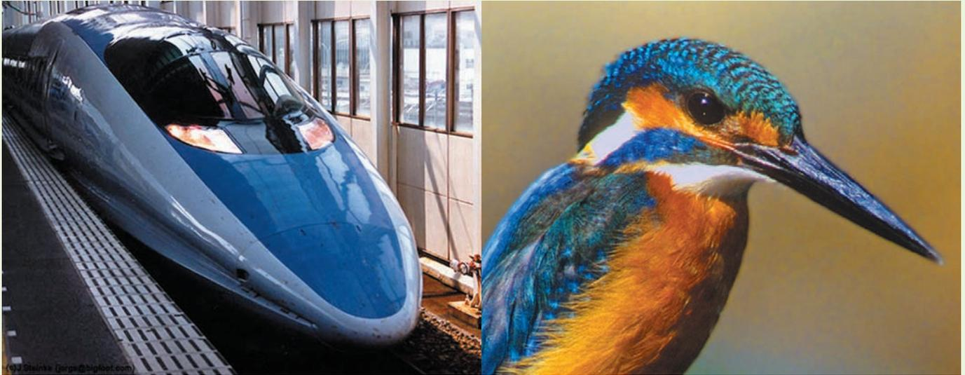
The design features of Japan's Shinkansen 500-Series exemplifies biomimicry in action. Its overhead pantograph sports serrations were modeled on the design of owl plumage to reduce air resistance noise, and the air piercing nose cone design was inspired by the kingfisher's beak. From the Swiss-Japan Assoc. for Engineers and Scientists.
