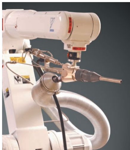
The new Cold Spray coating is still robotically applied, but at much lower temperatures. CSIRO
