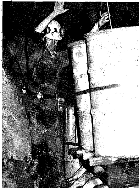
Samples of mine fill being placed to cure underground in 44-gallon drums.
