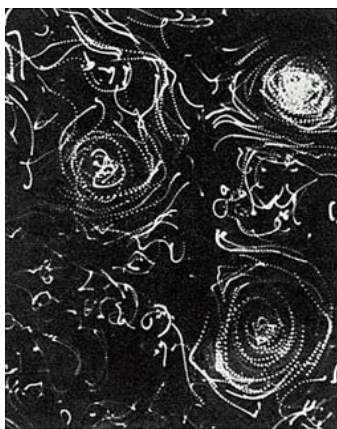
This photograph shows how polystyrene beads moved in eddies that formed in the water bath on the rotating turn-table.
