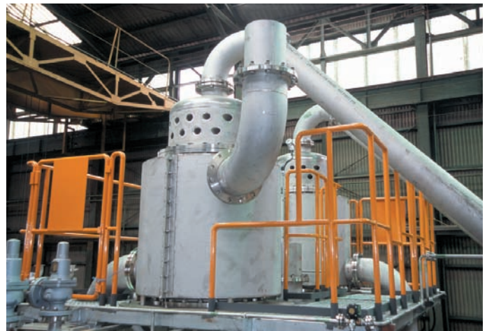
The catalytic converter of Ozmotech's promising ThermoFuel system. Ozmotech
