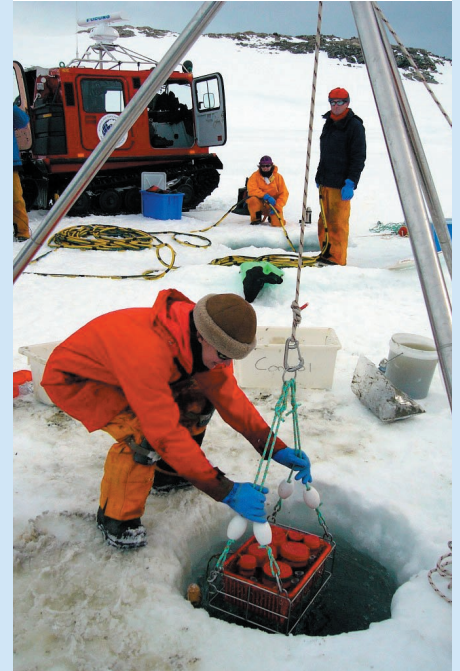
Dr Belinda Thompson retrieves a tray of sediment core samples collected by divers underneath the sea ice. The samples will be analysed for their chemical, microbial and biological composition. In the background, expeditioners watch the air lines to the divers. Shane Powell, Australian Antarctic Division, © Commonwealth of Australia
