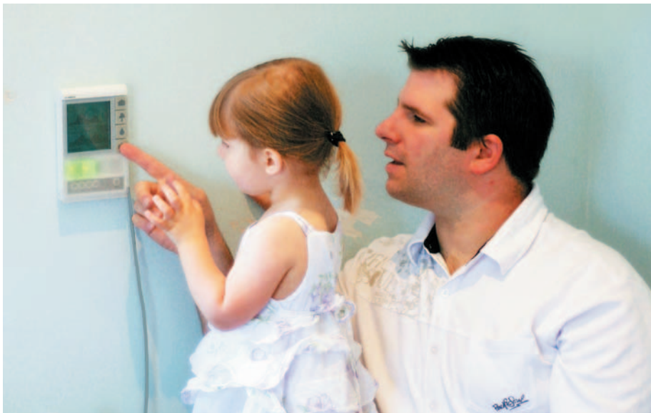
Smart meters provide real-time information on household energy use and estimated greenhouse gas emissions and could also advise, for example, half-hourly fluctuations in the price of energy to encourage low use during peaks. AMPY Email Metering
