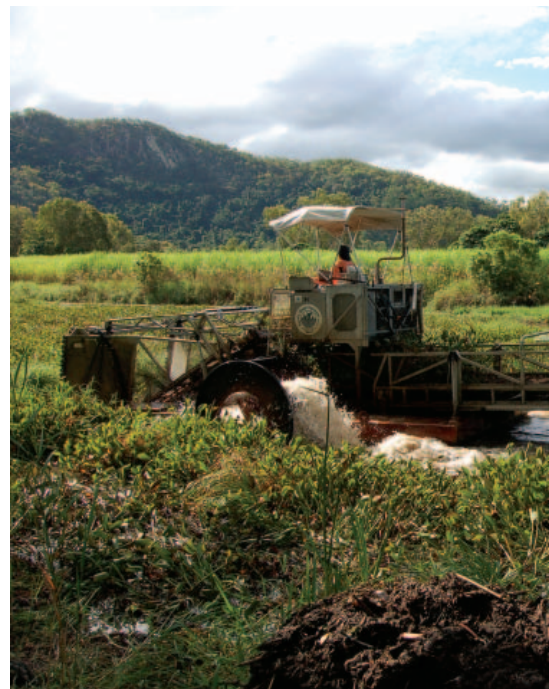
The paddle-powered harvester carving a track through the thick weed mat, helped by small punts. Vern Veitch
