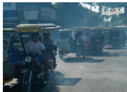
Each of the 1.3 million two-stroke motorcycle and tricycle engines in the Philippines produces an emissions load equivalent to 50 conventional cars. Envirofit
