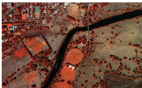
An aerial colour data image of riparian vegetation, houses and the sprinkler distribution impacts on lawn health on an irrigated oval in Perth. CSIRO
