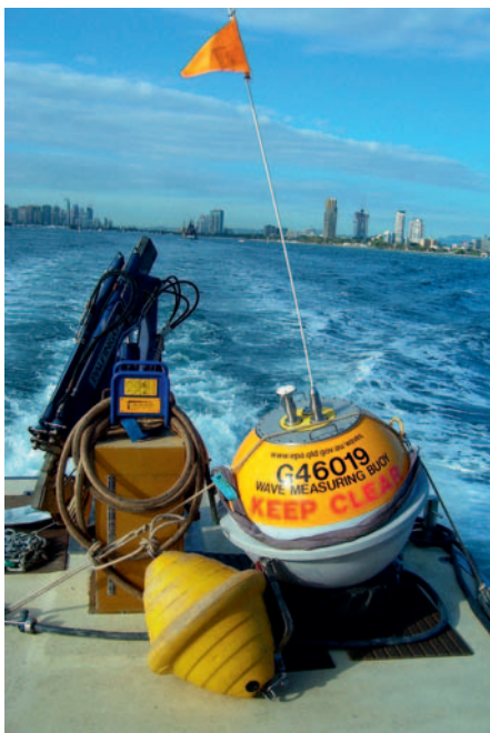
A wave-rider buoy being transported out to sea to begin recording swell events off Queensland. Courtesy of the Environmental Protection Agency, Queensland
