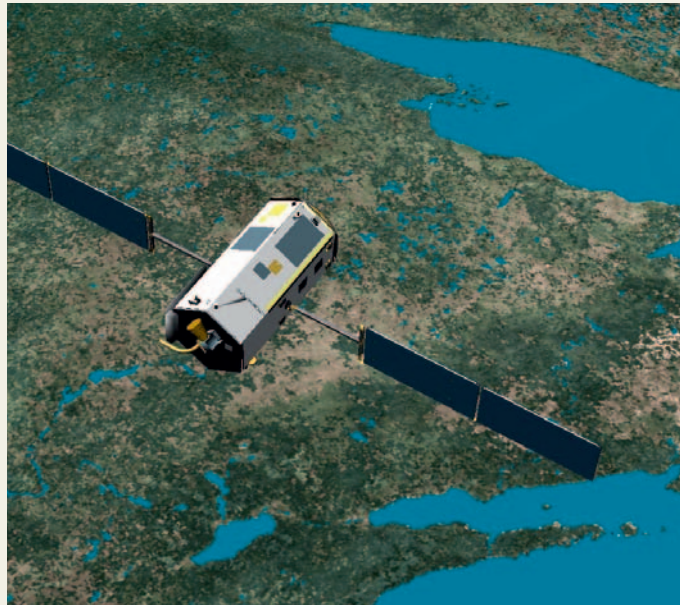
The new Orbiting Carbon Observatory will provide the most accurate maps to date of carbon dioxide sources and sinks globally. NASA
