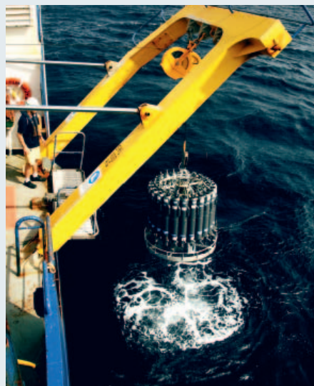
Deployment of an instrument from the Southern Surveyor that both samples sea water and measures conductivity (salinity), temperature and depth. Richard Arculus/ANU
