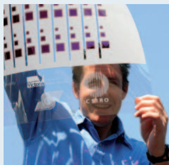
CSIRO researcher Dr Scott Watkins with a sheet of the thin-film polymer solar cells. Tracey Nicholls, CSIRO
