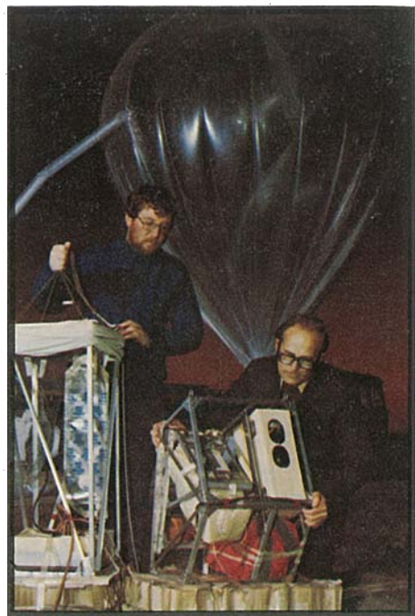
Members of the CSIRO team prepare instrument packages for a balloon of the type they plan to use to obtain stratospheric air samples for fluorocarbon measurements.
