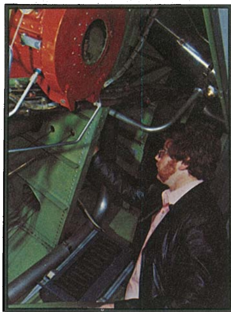
A CSIRO air-sampling pack is installed in an aircraft.
