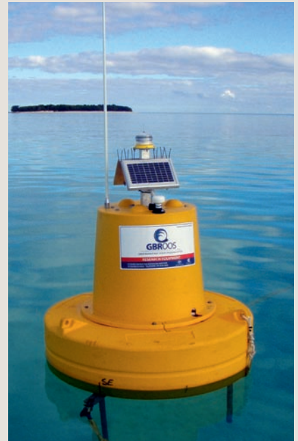
One of the sensor floats that makes up the IMOS sensor network at Heron Island, infrastructure which forms part of the Facility for Automated Intelligent Monitoring of Marine Systems (FAIMMS).
