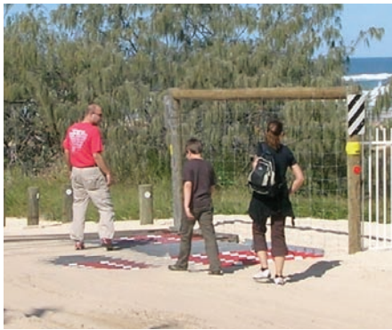
At Eurong village, tourists wilfully disregard QP&WS signs and walk across an electrified grid which has filled with sand. Nick Alexander
