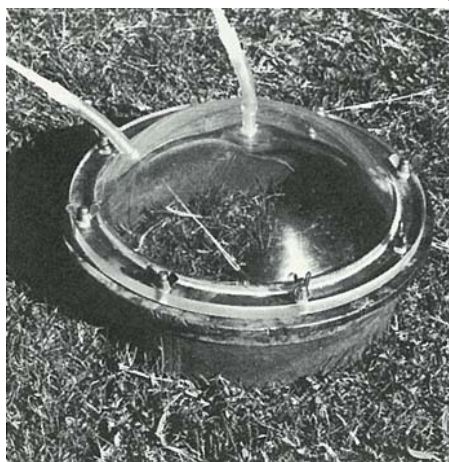
Chamber for measuring emissions of nitrous oxide from soil.
