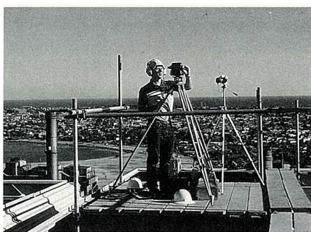
Mr Tony Eccleston atop Newport power station with a theodolite to fix the aircraft's position.
