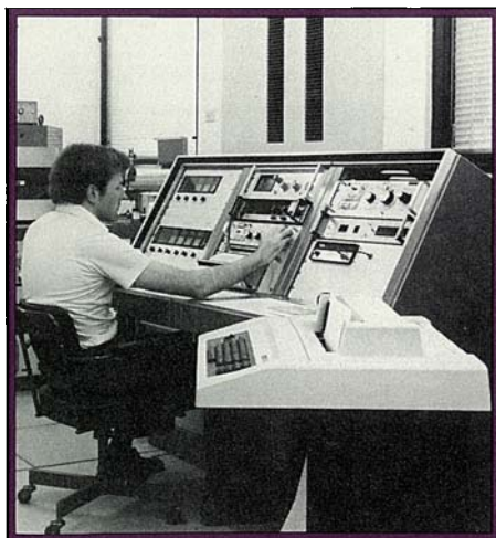
This mass spectrometer was used to examine the 'fingerprint' of lead isotopes. Lead from petrol was identified in soil samples in the Adelaide hills.
