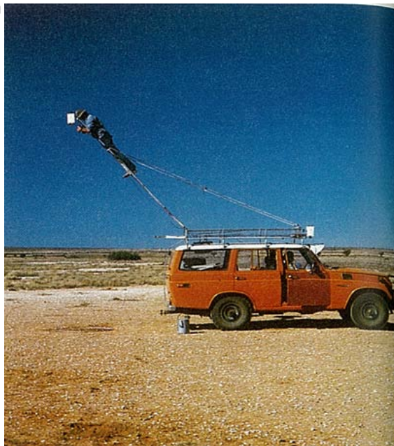
A radiometer, by picking up the same reflected wavelengths as Landsat, helps scientists to calibrate the satellite's images.
