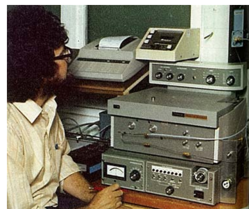
Instruments for measuring the minute concentration of methane in the air. A gas chromatograph equipped with a flame ionization detector is the heart of the system.
