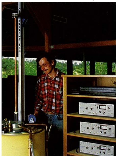
A researcher using the rock magnetometer to measure a specimen's magnetism.
