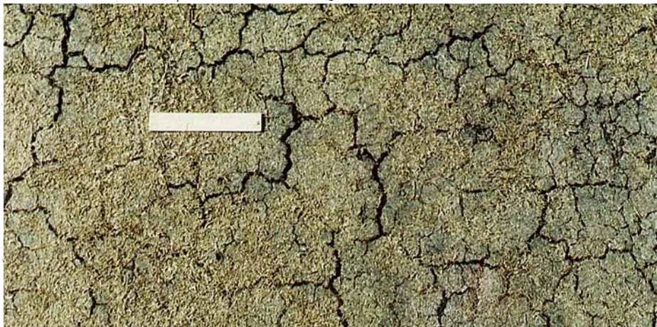
The old wicket in poor condition. Below: a close-up of some of the cracks, with a scale 150 mm long.
