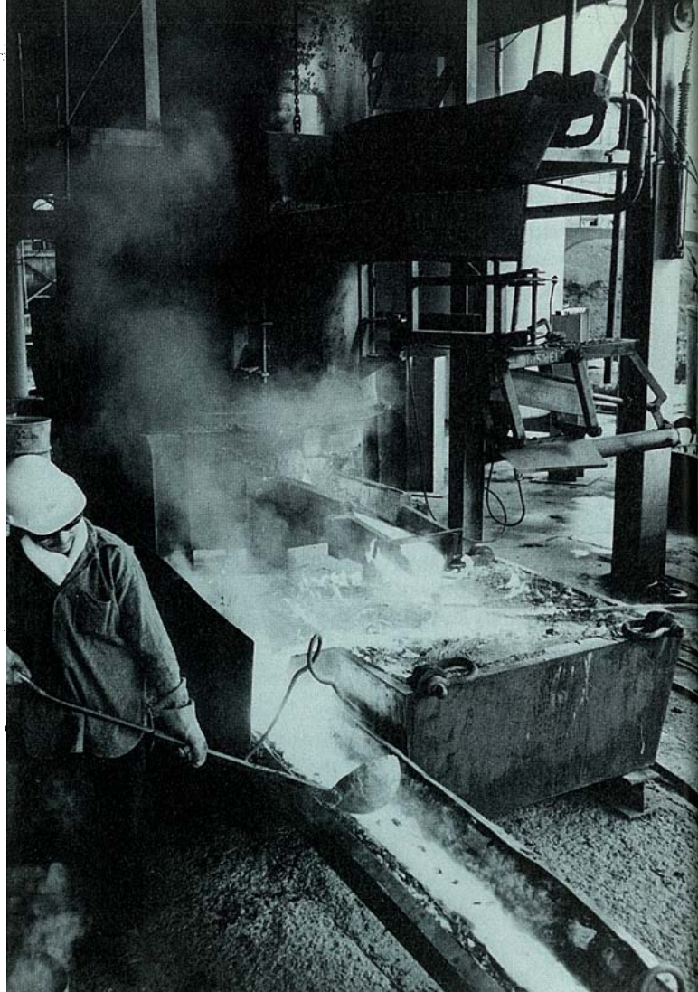
Sirosmelt at work. The products of slag reduction flow from a furnace at Associated Tin Smelters.
