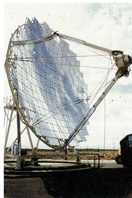
A parabolic dish developed by Ford Aerospace in California with an engine under test at the dish's focus.
