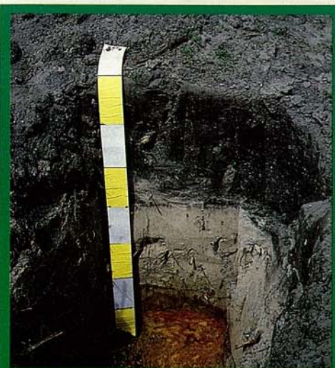
The soil layers of a Tasmanian study site at Grove Sand. The top darker grey layer contains large amounts of copper and lead; the deeper thin brown layer (50–60 cm depth) contains most of the arsenic. Each segment in the tape represents 10 cm.
