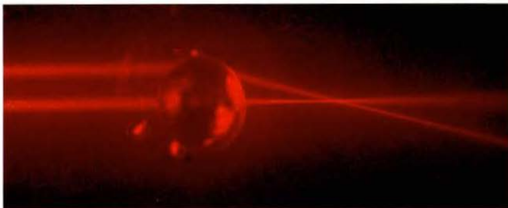
Laser beams focused by a rat-eye lens.
