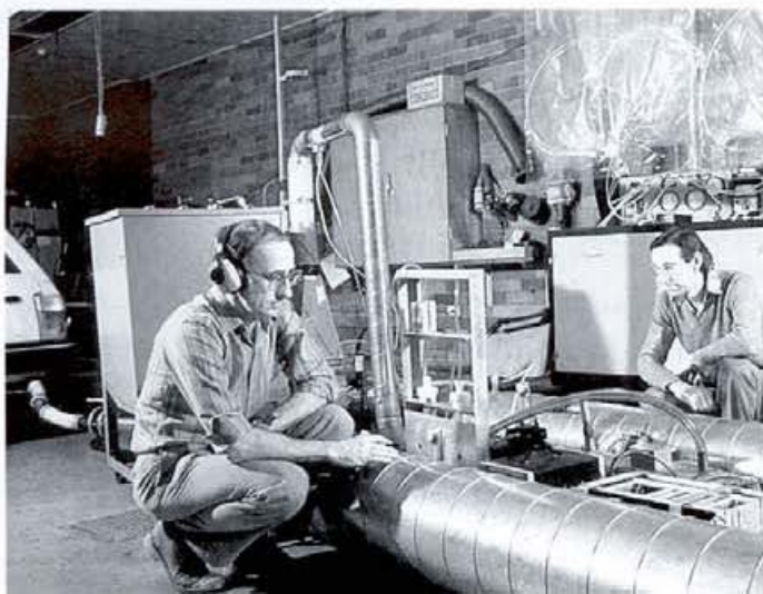
The dynamometer coupled to a test car.
