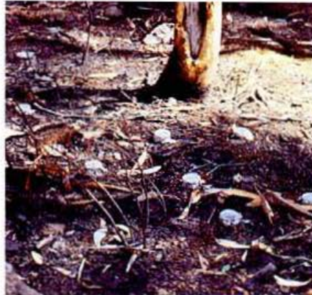
The small white-capped containers are used to measure nitrogen mineralization after a burn.
