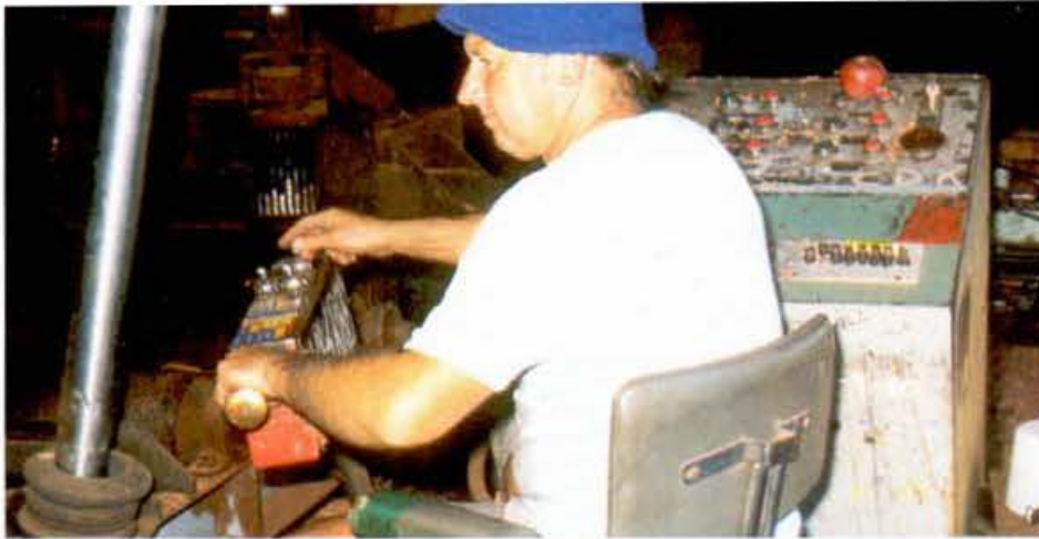
A resaw operator with the joystick and console controls that he has to operate up to forty or more times per minute throughout the working day.
