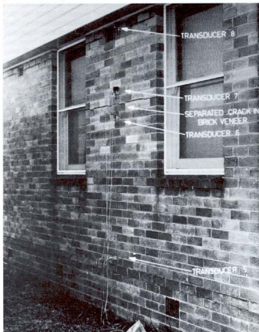
A brick-veneer wall magnifies ground vibration
