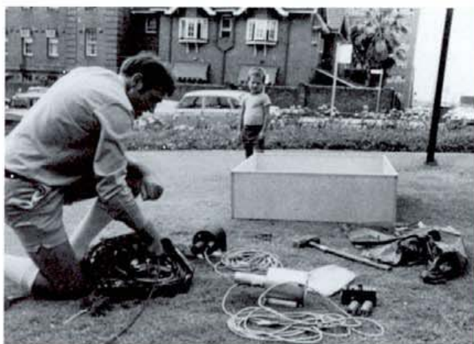
Setting up an array of seismometers next to Newcastle Hospital to measure ground vibration from nearby blasting.
