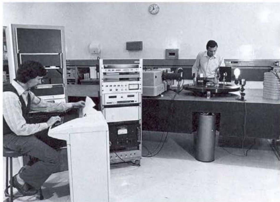
In the CSIRO spectro-radiometric laboratory. The researchers are preparing to test the UV output of a mercury-vapour street lamp.
