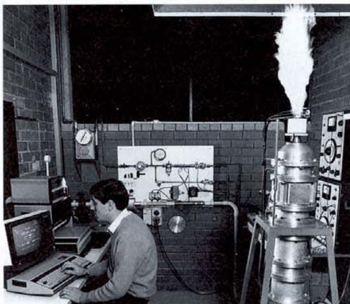
Scientists used a scale-model burner to find ways of reducing the noise of much larger industrial units.
