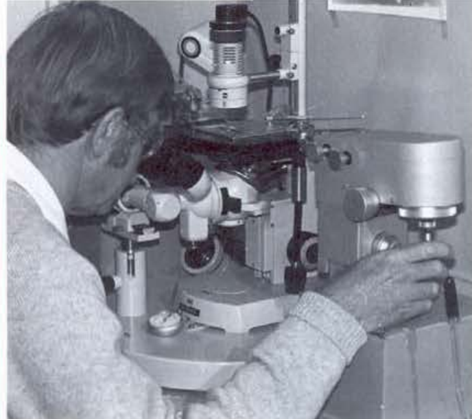
Dr Hill manoeuvres the micro-manipulator while watching his progress through the microscope. In this way he can literally cut open the nucleus of a living cell.
