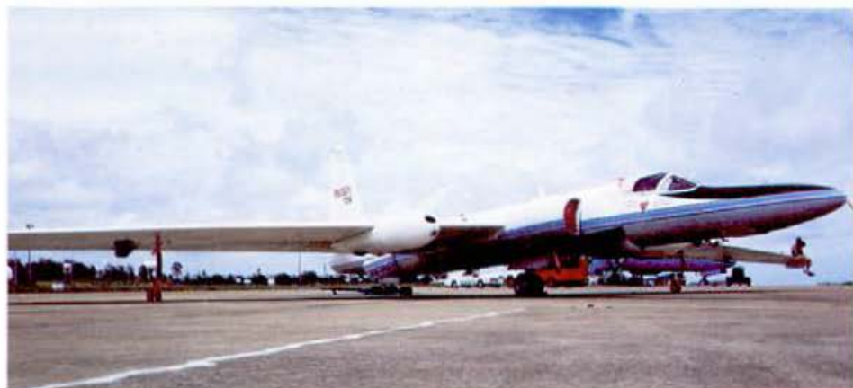
The ER-2 high-flying aircraft that went into the Antarctic stratosphere to take samples and analyse the chemical content of the air there.
