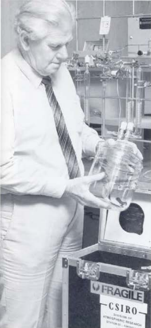
Inside the Cape Grim laboratory, Dr Francey extracts carbon dioxide from air piped down from the rooftop.
