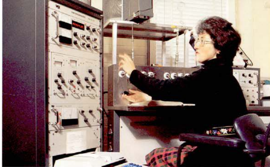
Helen Goodman uses a mass spectrometer to measure carbon dioxide isotopes.
