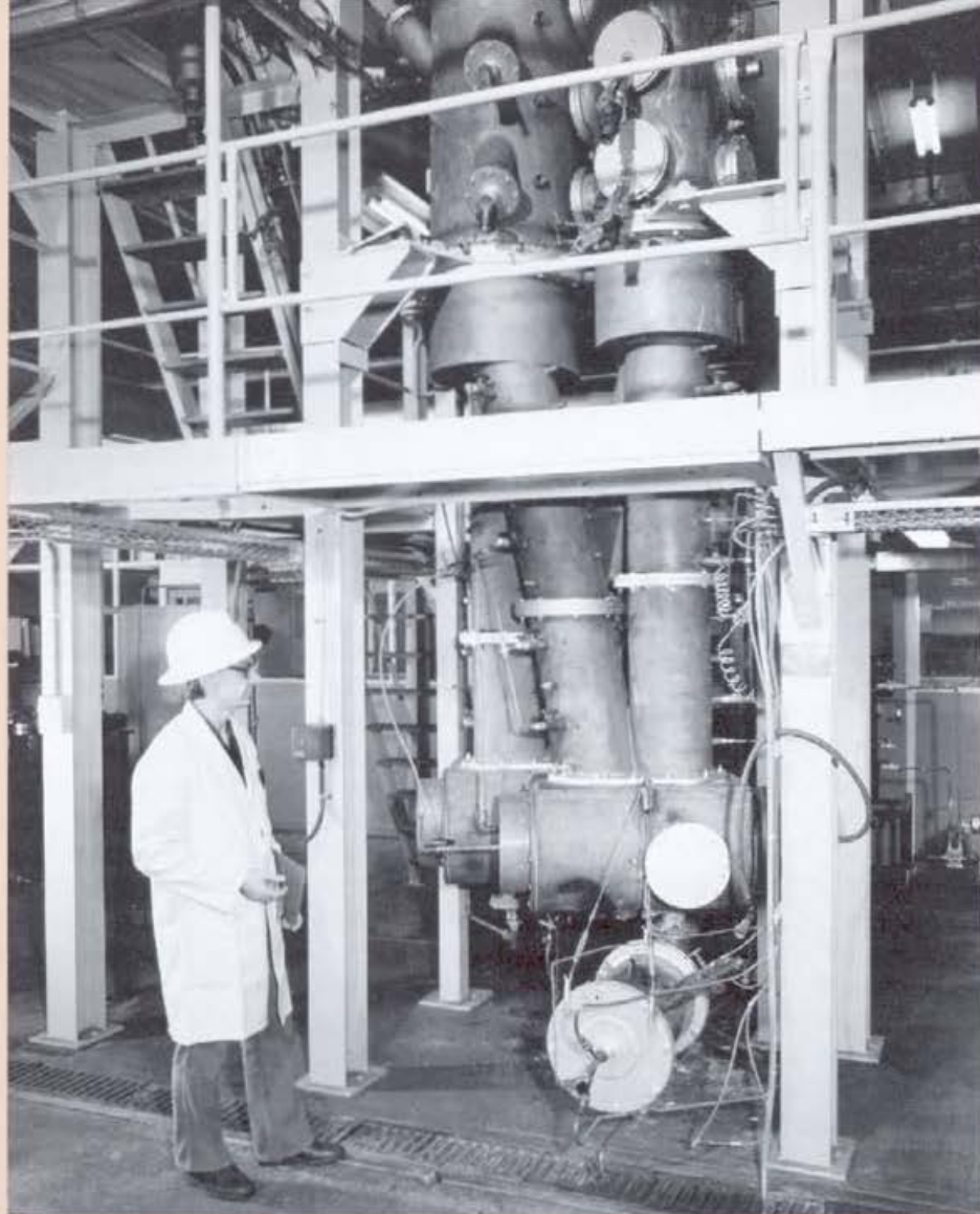
This rig for flash pyrolysis studies can, each hour, turn 20 kg of coal into char and tar.
