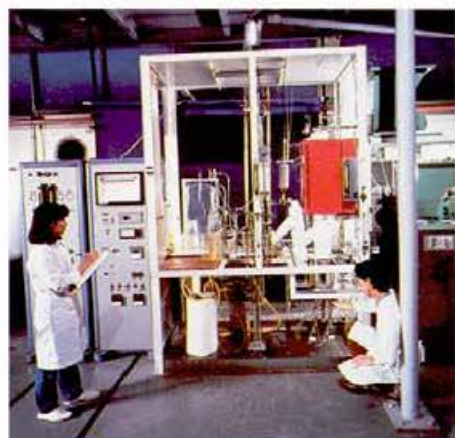
An experimental rig used by CSIRO scientists to study the pyrolysis of oil shale.
