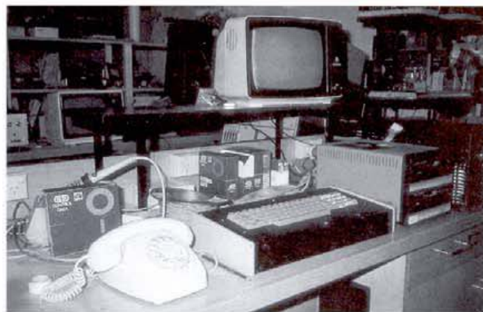
From mound to modem: signals about temperature in the forest termite mound are relayed by telephone through the modem and in to the laboratory computer.
