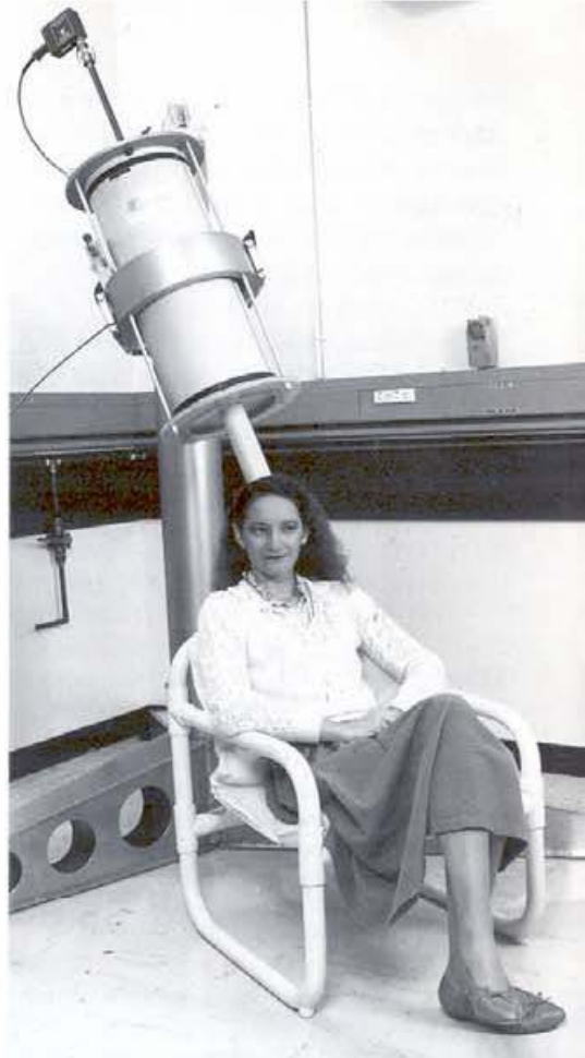
A biomagnetometer made by CSIRO can detect the very weak magnetic fields produced by nerve impulses in the brain. This one uses a superconducting detector cooled by liquid helium, but work with 'warm' superconductors could lead to a cheaper liquid-nitrogen-cooled version.
